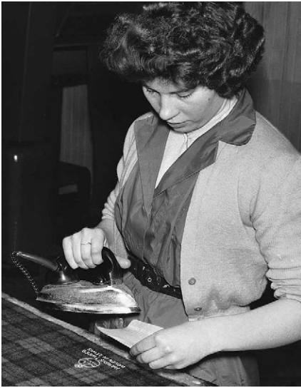
Figure 0.2. Stamping of the Orb trademark (pre-1969, n.d.). Photo © Harris Tweed Authority, used with permission.
